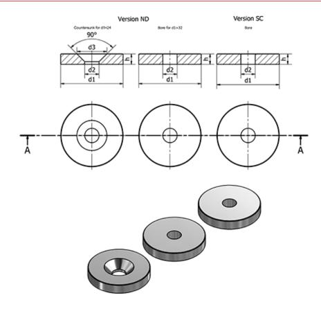
$\begin{array}{lll} d1 & = 56 \\ d2 & = 15 \\ d3 & = - \\ h & = 6 \\ Nominal adhesive forces in N = 230 \\ Weight in g & = 102 \\ \end{array}$
